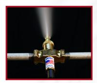
Model: Fogging (directed spray) Droplet size: 20 – 60 microns Liquid viscosities up to 1100 cP.
