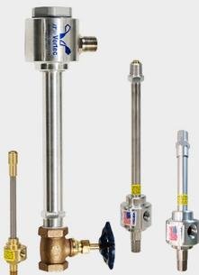
Vortex tubes produce up to 6000 BTU/hr (1757 watts) of refrigeration and temperatures as low as -40 deg to solve a variety of industrial spot cooling and process cooling needs. With no moving parts, a vortex tube is highly reliable and inexpensive; and requires no electrical connection at the cooling site. Vortex tubes cool instantly, relying on compressed air spinning in the tube to separate the air into cold and hot air streams.
