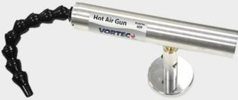
Hot Air Guns are used where milder heat is needed as compared to an electric heat gun. It is ideal for pre-heating of parts, processes and solutions, with an output flow rate of 2-8 scfm; and is also widely used for softening adhesives, rubber and vinyl, and accelerating drying. The hot air gun requires no electricity at the target, and uses only filtered compressed air to generate fully adjustable temperatures up to 200 deg F.
