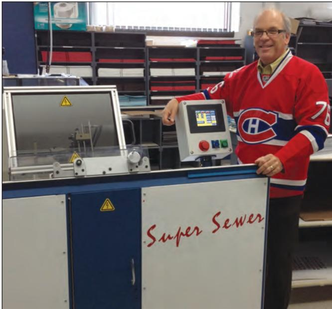
**Super Sewer™ side sews book blocks up to half inch thick at 600 per hour utilizing Vortec's Thread Guard™ needle cooler.**
